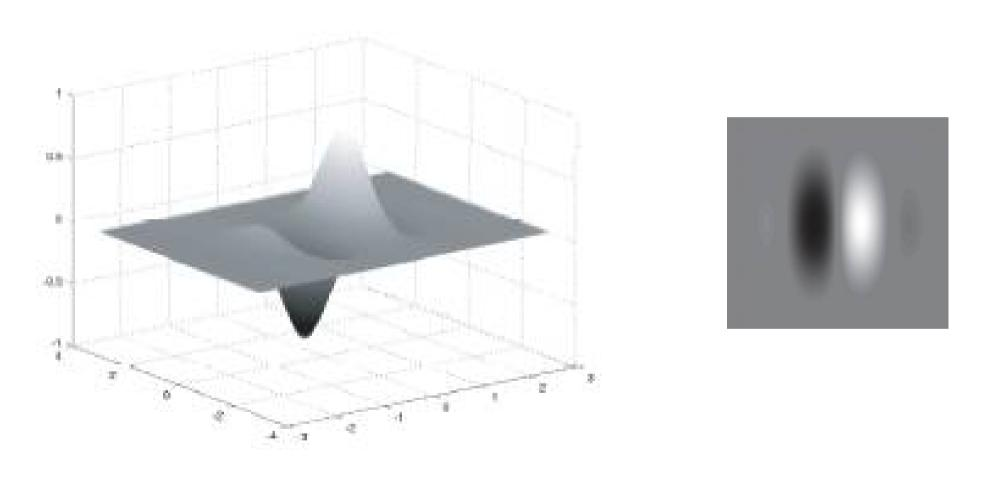
Simple cells can be modelled as derivative of a Gaussian
