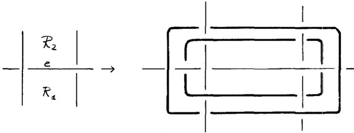
Fig. 53. How to remove multiple adjacencies along edges.
