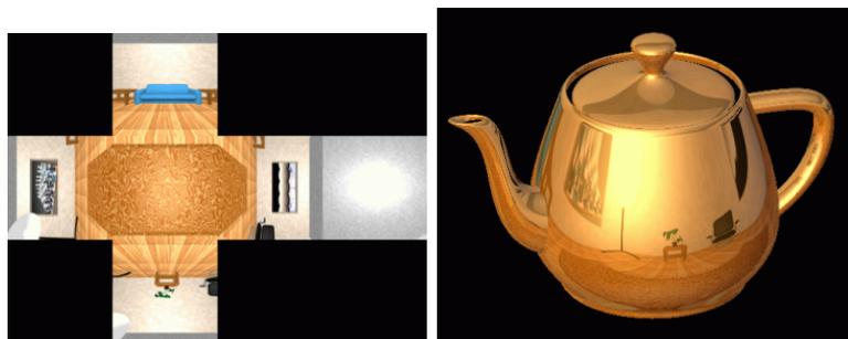
Figure 7.32: Environment mapping cubico
