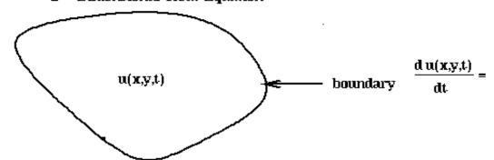
$$\frac{d u(x,y,t)}{dt} = C \left( \frac{d^2 u(x,y,t)}{d x^2} + \frac{d^2 u(x,y,t)}{d y^2} \right)$$
