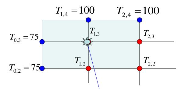
$$T_{0,3} + T_{1,4} + T_{1,2} + T_{2,3} - 4T_{1,3} = 0$$
