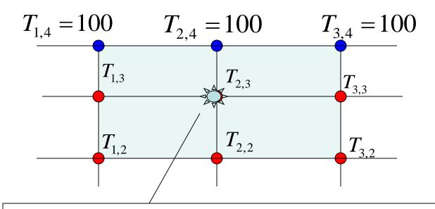
$$T_{1,3} + T_{2,4} + T_{3,3} + T_{2,2} - 4T_{2,3} = 0$$
