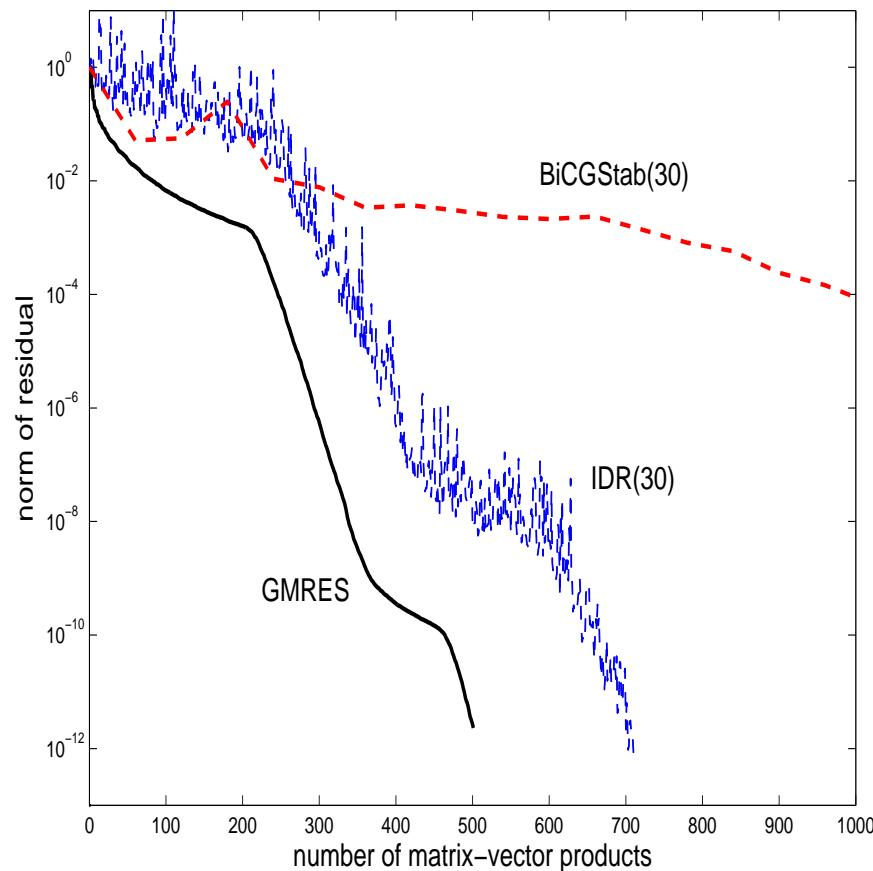
CPU Time: GMRES = 24 secs, IDR(30) = 2.58 secs, BiCGStab(30) = 20 secs
