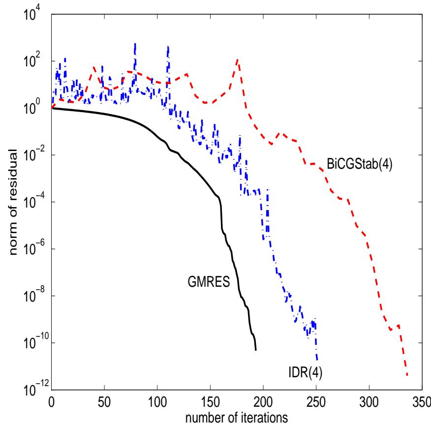
CPU Time: GMRES = 3.65 secs, IDR(4) = 0.22 secs, BiCGStab(4) = 0.32 secs
