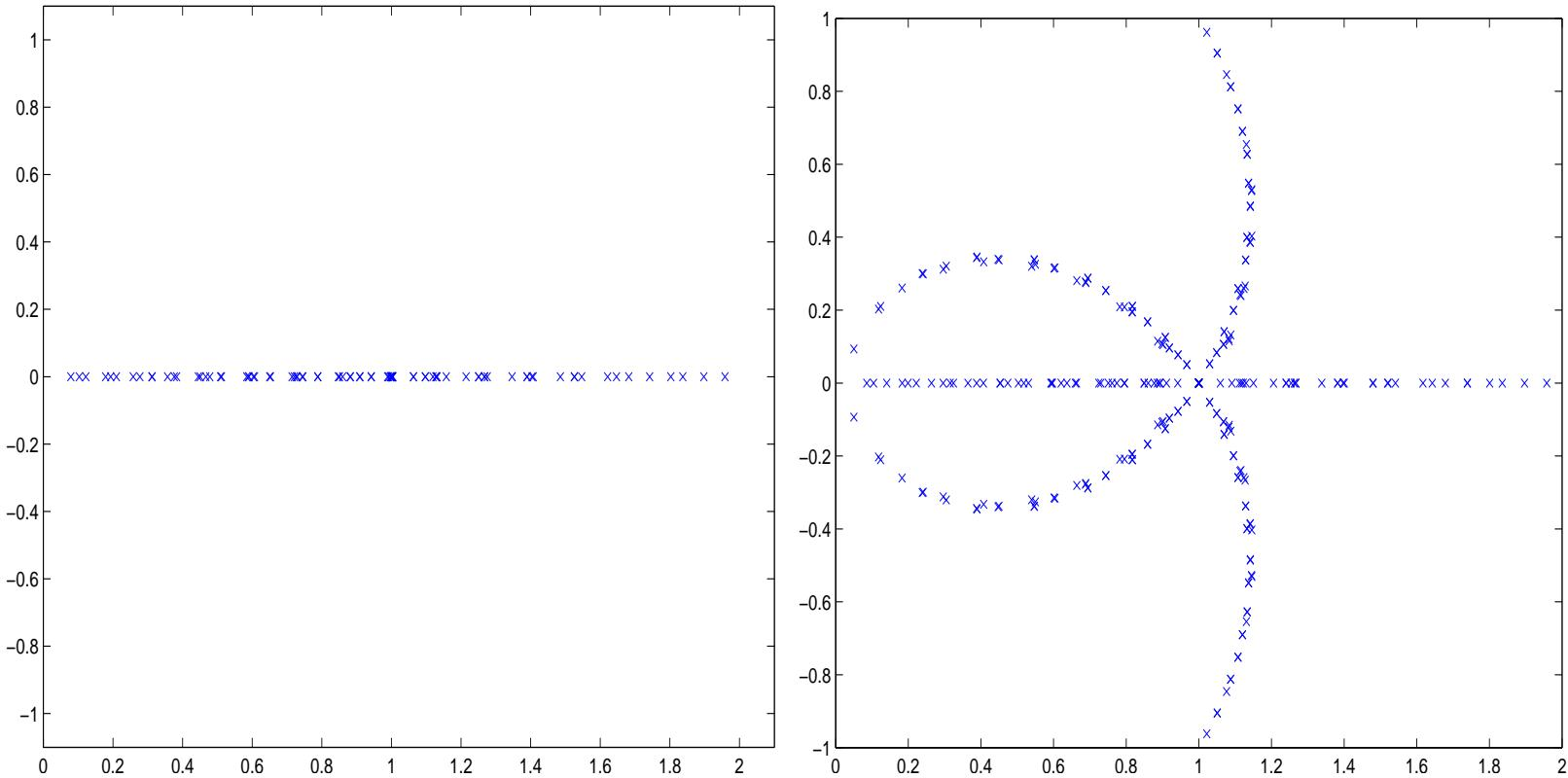
$$\|BB^T - S\|_\infty \approx 0.5\|BB^T\|_\infty \quad \tilde{A} = \text{diag}(A), \quad S = \text{diag}(B\tilde{A}^{-1}B^T)$$
