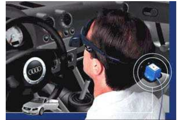
3D-BIRD mounted on Sony LDI-100 HMD, Audi TT Coupe virtual interior and exterior environment courtesy Eon Reality, Sweden.
